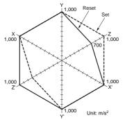
Sample: G6BK-1114P-US Number of Relays: 12 pcs Test Conditions: The value at which malfunction occurred was measured after applying shock to the Shock direction test piece 3 times each in 6 directions along 3 axes. Standard value: (Coil) 300 m/s<sup>2</sup>
